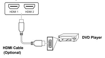
When the HDMI cable is connected, connecting the audio cable is not necessary. However, it is necessary to do so if a HDMI to DVI cable is connected.
