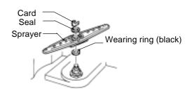
2) After the sprayer is taken off, wash out the adhered matters completely.
