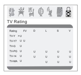
Note: You can press CH(+/-) buttons to go up and down the menu, then press VOL(+) button to select "B" (block channel) or "U" (unblock channel).
