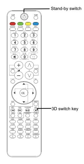
Press the 3D switch key on the remote control to call out the prompt menu. (See Fig. 1 below)
