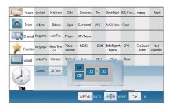
□ **Current Time**: The current time is calculated from the moment upon turning the TV on. At first, check whether the time indicated on the TV's clock is consistent with the standard time of your time zone; if not, adjust the clock as follows:
