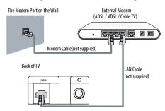
• You can attach your TV to your LAN by connecting the LAN port on the back of your TV to a router. which is connected to an external modem. Use a Cat 5 cable for the connection. See the diagram below:
