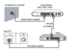
• Depending on how your network is configured, you may be able to attach your TV to your LAN by connecting the LAN port on the back of your TV directly to a network wall outlet using a Cat 5 cable. See the diagram below. Note that the wall outlet is attached to a modem or router elsewhere in your house.
