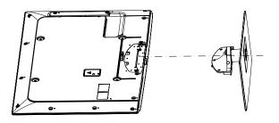
3.Push the stand onto the  $TV_{\,\circ}$
