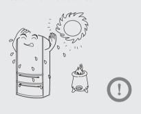
The refrigerator should be placed in a wellventilated place. A space of at least 20cm above and 10cm around the refrigerator is recommended.
