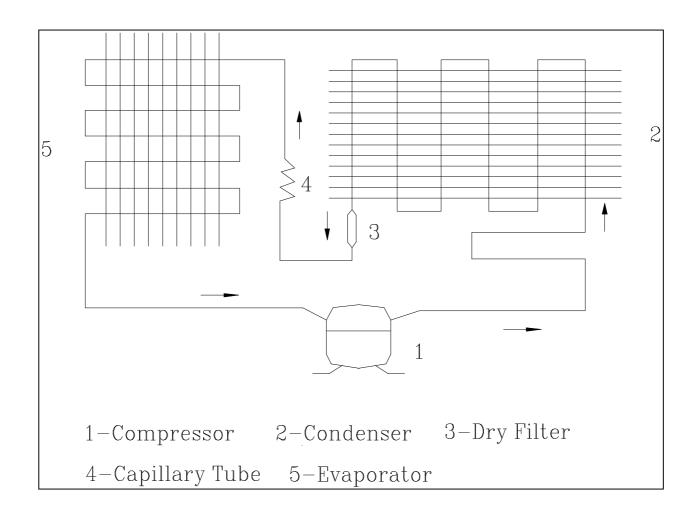
The refrigeration system of direct cooling single-system freezers belongs to the category of a single-temperature and single-control refrigerating system with only one evaporator and is controlled by a single temperature control.
