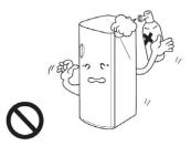
When cleaning the freezer, do not use water to wash the freezer; do not use hard bristle brush, wire brush to clean the freezer.
