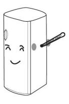
As the freezer use the back condenser surface for heat radiation so the temperature there would be high. It is a normal situation.
