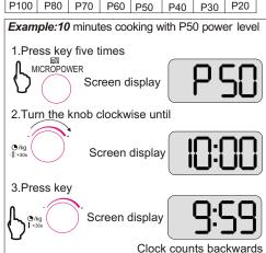
Note:1. The power level is displayed in the percent. With each pressing of the key MICROPOWER the power level reduces from p100 to P80 to P70to P60to P50 to P40 to P30 to P20 then start again from P100.
