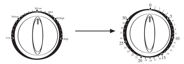
**Note:** As soon as the timer is turned, oven will start cooking. When setting timer for less than 2 minutes, turn timer past 2 minutes and then return to correct time. When time has elapsed, a bell will ring and the unit will turn off.
