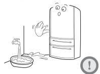
The refrigerator should be placed in a well-ventilated place not far from a drink water source. A space of at least 20cm above and 10cm around the refrigerator must be kept.
