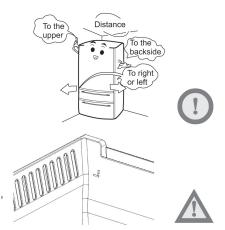
The appliance must be positioned so that the plug is accessible.
