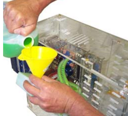
Figure 4: If possible or desired, you can also fill the reservoir outside of the chassis. Tipping it steeply at an angle will allow you to fill-it up at the maximum operating level as shown figure 5. Do not forget to close the fill-cap before you re-install the unit into the drive bay!
