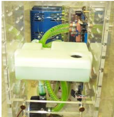
Figure 3: The minimum operating fluid level is at the mould parting line.
