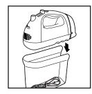
The Snap On Case keeps attachments with the mixer for easy storage. Place attachments into case. Align tab at the back of the accessories case with the corresponding notch on the bottom of mixer. Press case on mixer until it snaps into place.
