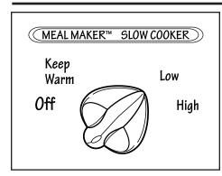
The Control Knob on the slow cooker offers Low and High temperature settings for cooking. The Keep Warm setting is for holding the prepared recipe at a perfect serving temperature.
