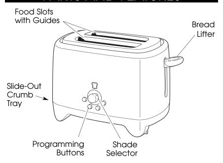
**Bread Lifter** – Push down the Bread Lifter to start the toaster. The Bread Lifter may be lifted up to stop toasting during a cycle.
