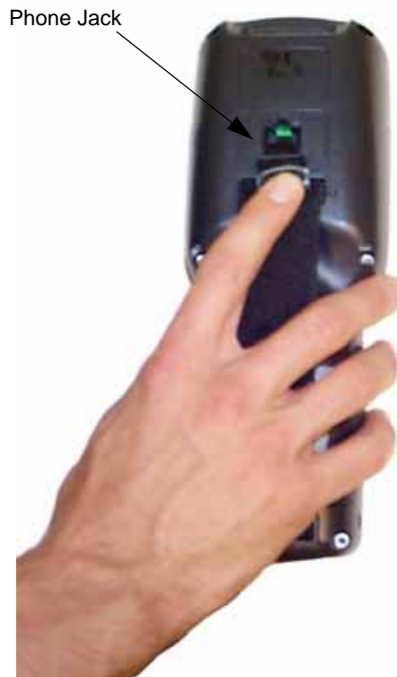
Phone Jack on rear of Dolphin 7400
