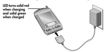
**Tip:** When your phone is on, the charge icon application while your VisorPhone charges. Note that your VisorPhone must be in your handheld while charging, and that it takes about 1.5 hours to fully charge the battery. It's time to recharge the battery when you observe one of the following:
