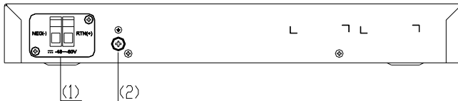
Figure 1-21 Rear panel of the S3100-8C-SI model supporting DC input
