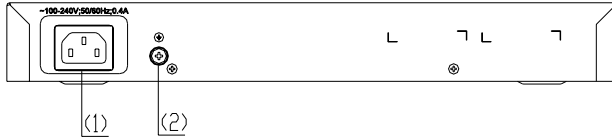
Figure 1-20 Rear panel of the S3100-8C-SI model supporting AC input
