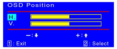
**OSD Position :** Press the **②** button to select the horizontal or vertical OSD position.
