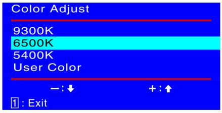
**Color Adjust:** To provide four preset color adjustments for improving brightness and color saturation: 9300K, 6500K, 5400K, and User Color. Press button ② to select the preset color.
