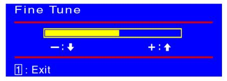
**Fine Tune :** To adjust the delay time of data and clock.
