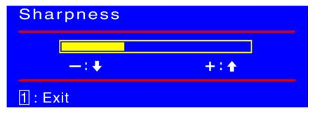
Sharpness: To adjust the clarity of a non-SXGA (1280x1024) signal. Press ▼ or ▲ button to adjust.
