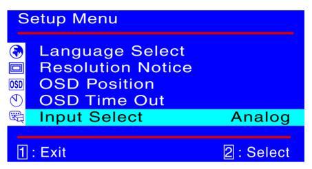
**Input Select :** When press Input Select change Input signal to Analog or Digital.
