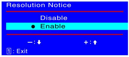
**Resolution Notice :** There is a OSD message of "For best picture quality change resolution to 1280 x 1024" displayed on the screen after 30 seconds Powering ON or changing mode to lower resolutions (640 x 480/ 720 x 400 / 800 x 600/ 1024 x 768), if the function was "enable". Above message would not display on screen if it was "disable".
