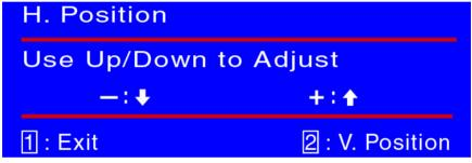
**H./V. Position:** To adjust the horizontal and vertical position of the video.
