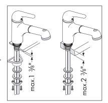
The spout should swivel equally to the right and to the left. If it appears to swivel more to one side than to the other, pivot the faucet body until the swivel is even.
