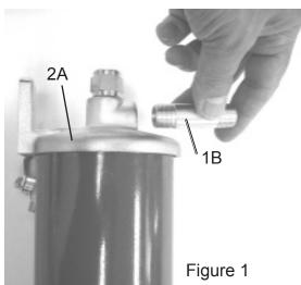
1. Remove the contents in the small plastic bag and locate Nipple (1B). Thread the Nipple (1B) into the side port of the Filter Cap (2A). You should use pipe thread seal tape or pipe dope (not included) on all threaded connections. See Figure 1.
