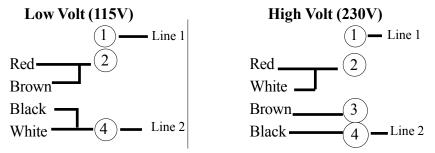
Rotation is CCW-OPE; to reverse either voltage interchange Red and
