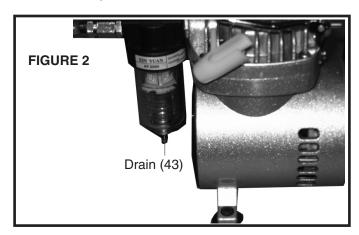
3. The Filter (42) cup will fill with moisture from air that flows through the filter. After each use, push the Drain (43) under the cup to drain off the moisture. See **FIGURE 2**.
