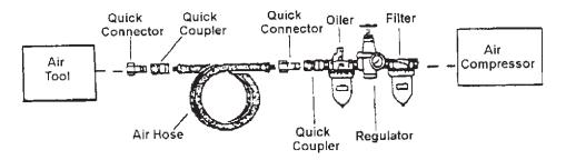
**Note:** Use pipe thread seal tape on all threaded connections.
