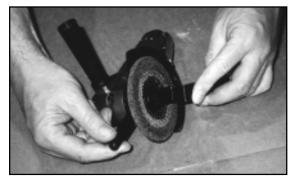
holes in the Disc Nut [1] and turn your wrist to unscrew the Disc Nut. Seeig.ig. A, right.
