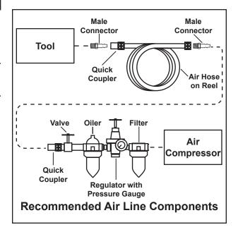
Incorporate an in-line oiler, shut-off valve, regulator with pressure gauge, and filter for best service, as shown in the diagram above. An in-line shutoff valve is an important safety device because it controls the air supply even if the air hose is ruptured.
