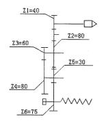
eg: request feed distance 8TPI Given: spindle gear Z=40
