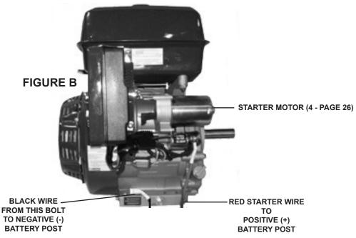
To provide battery power to the Starter Motor (4 - page 26), connect the BLACK (negative -) wire from the negative (-) post on the battery to the Bolt designated on the base of the engine. Then connect the RED (positive +) wire from the Starter Motor to the positive (+) post on the battery. (See Figure B.)
