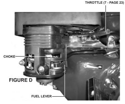
To start the Engine, turn the Fuel Lever to its "OPEN" position. Turn the Choke to its "START" position. Then turn the Throttle to the RIGHT to its "SLOW" position. (See Fig. D.) Note: If the Engine is already hot, keep the Choke in the "RUN" position.
