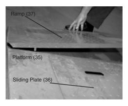
1) Place the Sliding Plate (36) onto the Platform (35) to cover the rear wheel removal opening.
