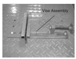
3) Clamp the front wheel of the motorcycle into the Vise Assembly to prevent movement of the wheel. For maximum safety, you should also stabilize the motorcycle using tie-down straps (not included).
