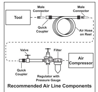
1. Attach an air hose to the compressor's air outlet. Connect the air hose to the air inlet of the tool. Other components, such as a connector and quick coupler, will make operation more efficient, but are not required.
