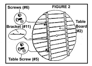
3. Attach the **Table Stand (#1)** to the **Brackets (#11)** on the **Table Board (#2)** using two sets of **Screws (#6)**. See **FIGURES 2 & 3**.
