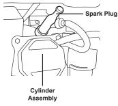
emery paper. If the white insulator is cracked or chipped, the spark plug needs to be replaced.
