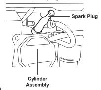
it using emery paper. If the white insulator is cracked or chipped, the spark plug needs to be replaced.
