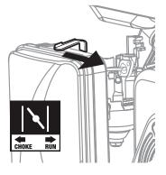
**NOTE:** Moving the Choke Lever too fast could stall the engine.
