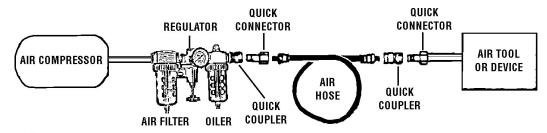
Connect the air tool, air hoses, filter, and oiler to the Compressor Air Outlet as illustrated below. Use pipe thread seal or Teflon tape on all threaded connections. The filter and oiler (not supplied) are recommended but not mandatory for operation.
