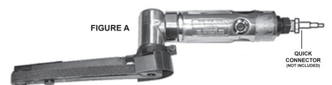
For best tool performance, you should incorporate an in-line water filter, regulator and oiler as shown in the illustration below. If an oiler is NOT used, it is recommended that you squirt 3 to 4 drops of pneumatic tool oil (not included) into the previously installed Quick Connector of the tool before each use. (See Figure B.)
