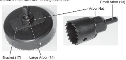
10. Remove Hole Saw from drilling tool chuck.
