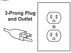
Your unit has a plug as illustrated above. The outlet used should look like the outlet illustrated above. Do not remove the grounding prong from the plug. If the plug will not fit the outlet, have a proper outlet installed by a qualified electrician.
