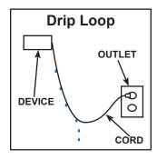
6. Use Drip-Loop to prevent water from accidentally entering the electrical power outlet. Use only with a GFCI outlet. See second paragraph in "Power Cord Safety" section of this manual.
