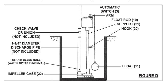
Do not attempt to reduce the discharge size below 1-1/4" as this will affect Pump flow and performance. A Schedule 40 PVC 1-1/4" diameter Pipe is recommended. (See Figure D.)
