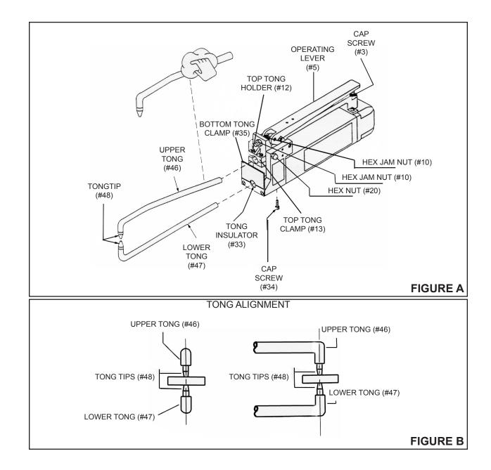
10. Retighten the four Cap Screws (parts #3, #11).
