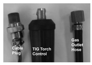
Connect the TIG torch control, cable 1. plug, and gas outlet hose as shown on page 12. Twist to lock in place.
