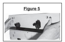
Step 3) The Swivel Pegs (#1) and Peg Supports (#5) can be placed into any hole in the Work Table top provide a block to secure and block your workpiece.
