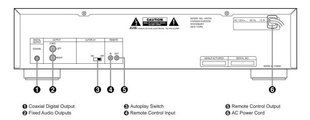
• Coaxial Digital Output: Connect this jack to the coaxial digital input of an external digital-to-analog converter for direct access to the digital signals of the HD720. DO NOT connect this jack to the standard audio inputs of any device.
