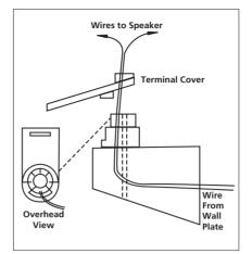
The bracket has two openings on top: a round screw hole, and an arc-shaped opening in front of it. The speaker cable should be threaded through the arc-shaped opening, not the screw hole.
