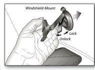
Do not install this device in any manner that impairs the safe operation of the vehicle. Do not install this device on any
