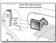
Installation of TMC antenna cable to receive traffic information
