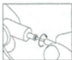
2. Firmly push the sharp tip of the filter tool into the center of the filter.
