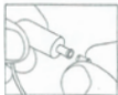
1. With your fingers, put the narrow end of a new filter into the end of the earphone. Be careful to put the open end in first so that the filter can be seen at the tip of the earphone. Gently push on the filter and snap it into the earphone. You should feel and hear it snap in place.
