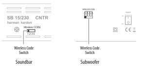
NOTE: The maximum wireless operating distance between the soundbar and subwoofer is approximately 50 feet (15.3m).
