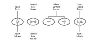
**Power Button:** When the soundbar is in the Standby mode (the Power Indicator is amber), press this button to turn the SB 15/230 system On. (The Power Indicator turns blue.) NOTE: When the soundbar is in the Standby mode, it will automatically turn On whenever it detects an audio signal at the Source 1 (analog) inputs.
