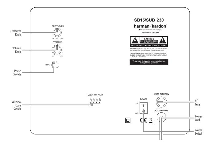
**Crossover Knob:** This knob adjusts the subwoofer's crossover between 50Hz and 150Hz. The higher you set the Crossover knob, the higher in frequency the subwoofer will operate and the more its bass will "overlap" that of the soundbar. This adjustment helps achieve a smooth transition of bass frequencies between the subwoofer and the soundbar for a variety of different rooms and subwoofer locations. See *Subwoofer Crossover Knob*, on page 9, for more information.
