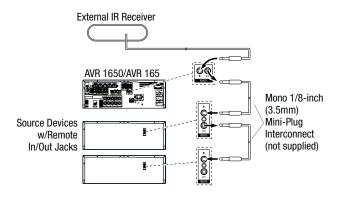
To control more than one source device through the AVR's IR Remote Out connector, connect all sources in "daisy chain" fashion, connecting each device's IR output connector to the next device's IR input connector, starting with the AVR.
