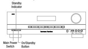
Unless you will not be using the AVR for an extended period of time, leave the Main Power switch set to "On." When the Main Power switch is turned off, any settings you have programmed will be preserved for up to two weeks.
