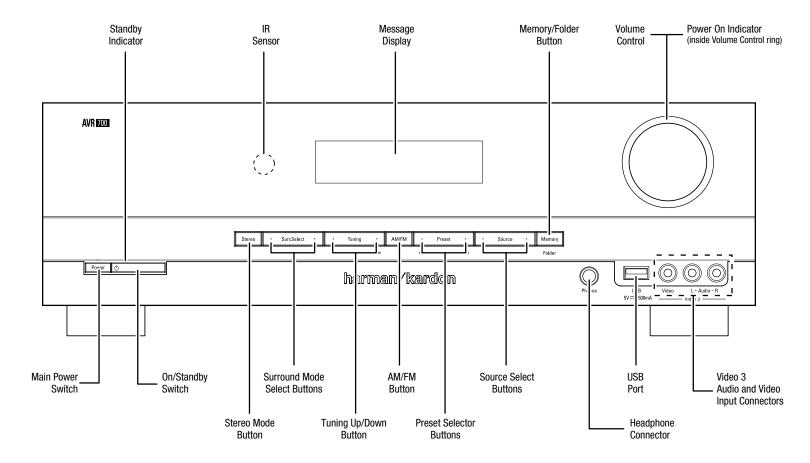
Main Power switch: This mechanical switch turns the AVR's power supply on or off. It is usually left on and cannot be turned on or off using the remote control.
