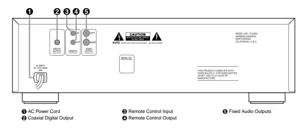
**O** AC Power Cord: Connect this plug to an AC outlet. If the outlet is switch controlled, make certain that the switch is in the ON position.
